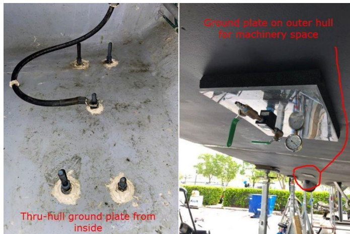
Fig 1: Hull Earth / Ground Plate (Courtesy of American Bureau of Shipping)
