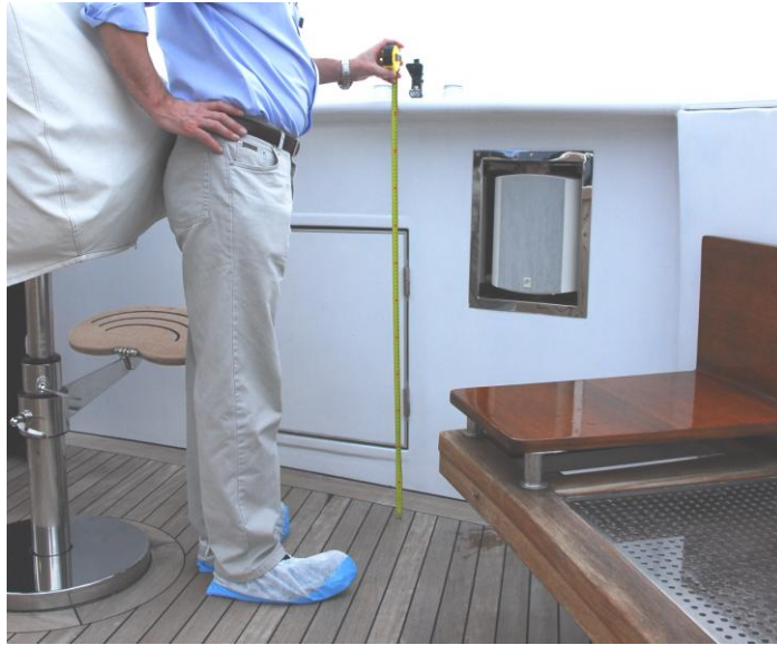
Figure 3 Forward bulwark on wheelhouse top. (1.145m height)
