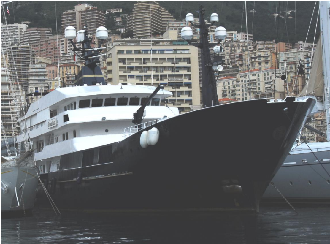
Figure 2 View of height from wheelhouse top to waterline.(approximately 12m)
