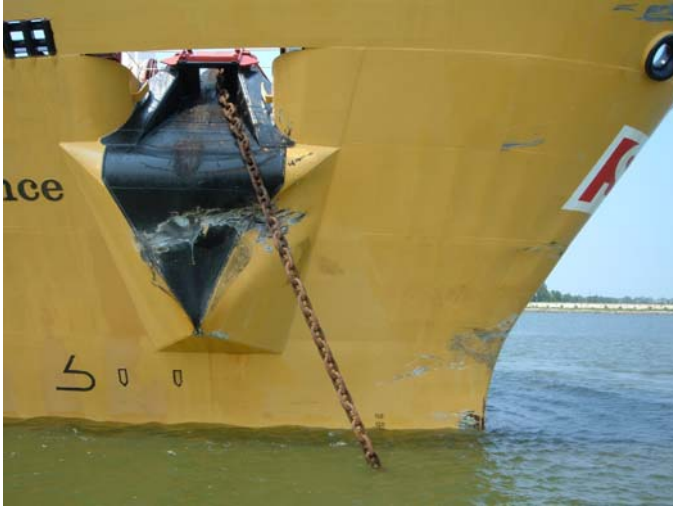
Fig 1: Area of contact in way of starboard anchor pocket.
