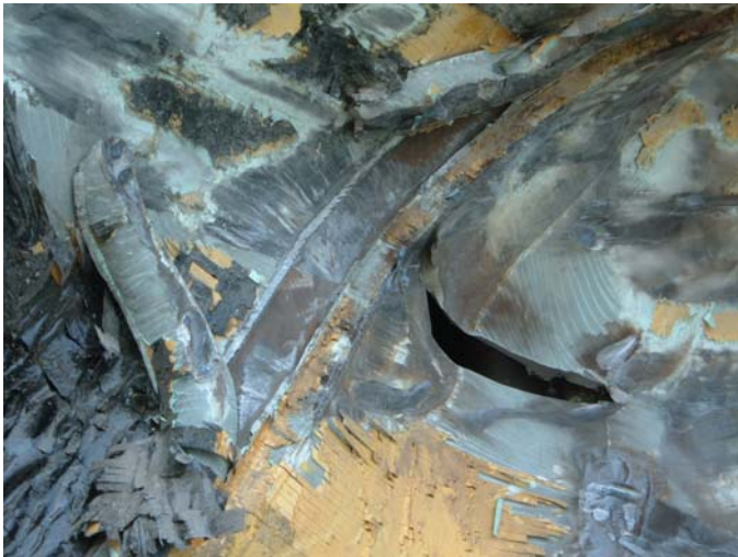
Fig 2: Detail of hole into fore peak
